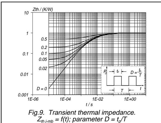
Silicon Diffused Power Transistor
