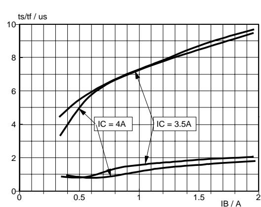
Fig.12. Limit storage and fall time.
