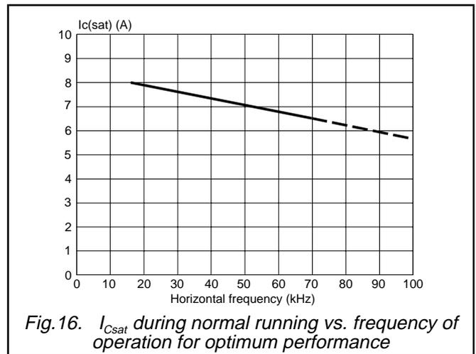
Silicon Diffused Power Transistor
