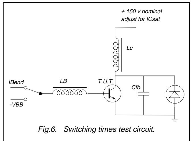
Silicon Diffused Power Transistor
