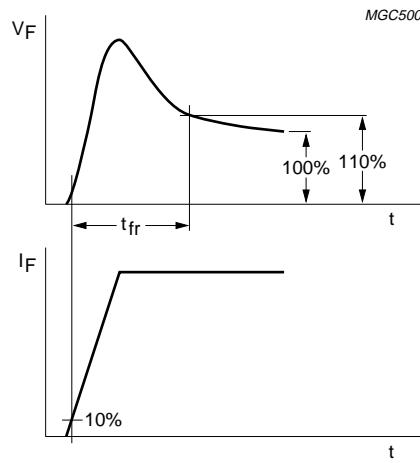
Fig.9 Forward recovery time definition.
