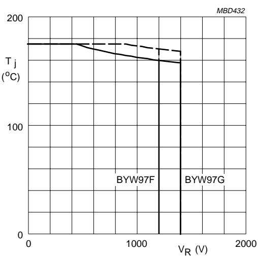
Fig.7 Maximum permissible junction temperature as a function of reverse voltage.
