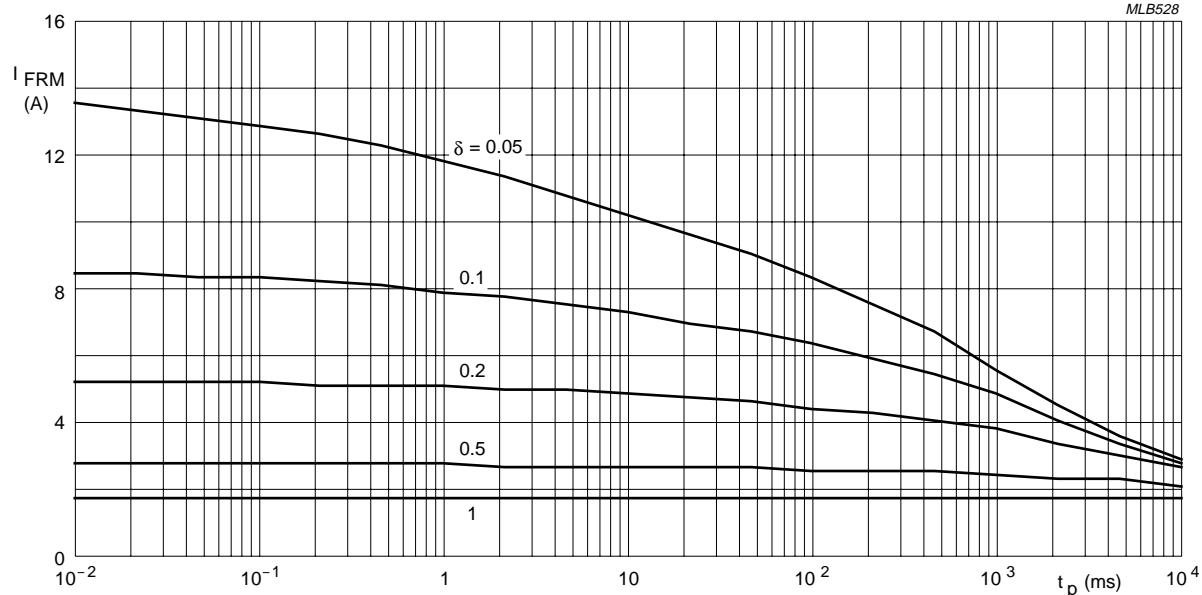
$T_{amb} = 55^\circ C$ ;  $R_{th\ j-a} = 75 \text{ K/W}$ .
