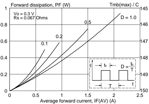
Fig.1. Maximum forward dissipation per diode
