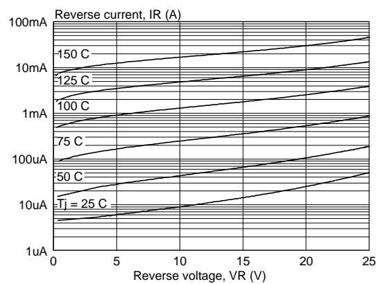
Fig.4. Typical reverse leakage current per diode;
