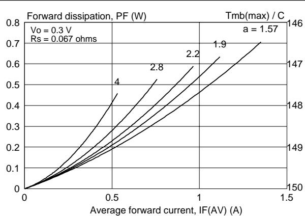
Fig.2. Maximum forward dissipation per diode
