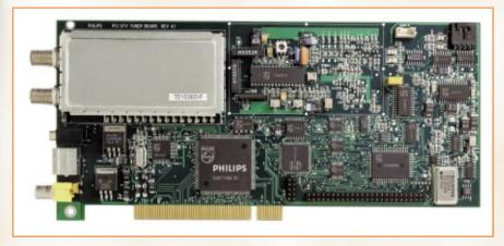
At the heart of Philips' Coney board are a number of very highly integrated, highlyfeatured ICs, essentially a single-chip solution for each core function.
