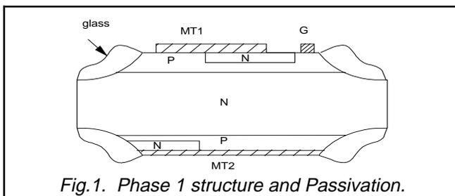
Fig. 1. Phase 1 structure and Passivation.
