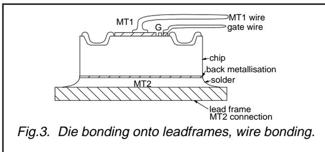
Fig.3. Die bonding onto leadframes, wire bonding.
