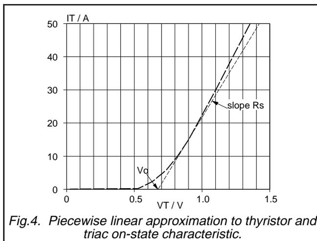
Fig.4. Piecewise linear approximation to thyristor and triac on-state characteristic.
