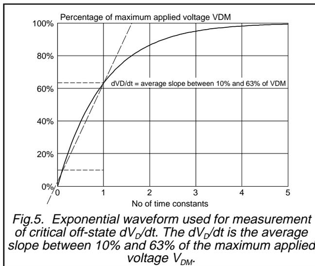
Fig.5. Exponential waveform used for measurement of critical off-state  $dV_D/dt$ . The  $dV_D/dt$  is the average slope between 10% and 63% of the maximum applied voltage  $V_{DM}$ .
