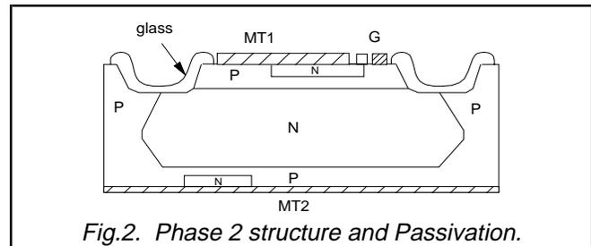
Fig. 2. Phase 2 structure and Passivation.
