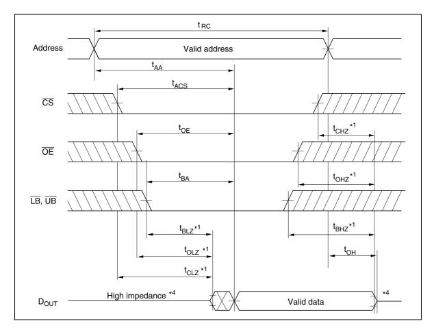
Read Timing Waveform (2)  $(\overline{WE}=V_{_{IH}},\overline{LB}=V_{_{IL}},\overline{UB}=V_{_{IL}})$
