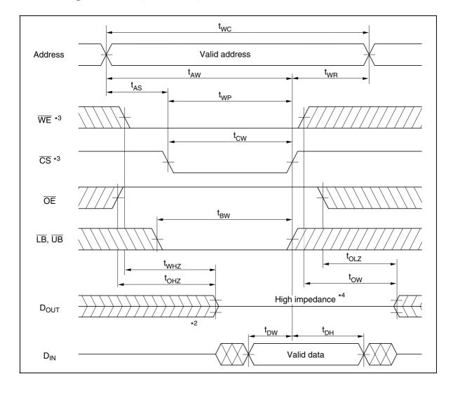
Write Timing Waveform (3) ( $\overline{LB}$ ,  $\overline{UB}$  Controlled,  $\overline{OE} = V_{H}$ )
