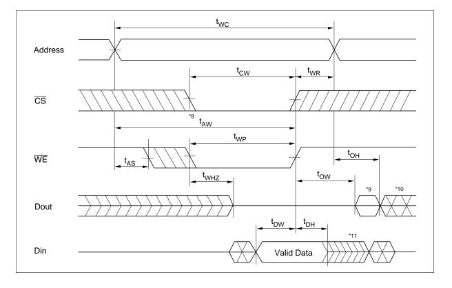
Write Timing Waveform (2) (OE Low Fixed)
