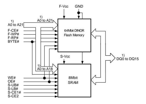
Note 1): In case of x8 organization, A-1 is added, and only Lower Byte data(DQ0 to DQ7) are assigned to I/O and Upper Byte data(DQ8 to DQ15) are High-Z.
