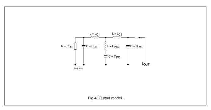
A second method in designing the matching circuit is to use the measured data in a dataset. This has the disadvantage that inconsistency in data will have a larger influence than when a model is used.
