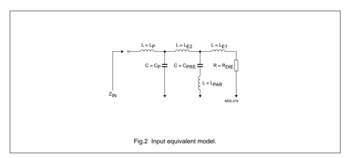
Apart from bandwidth considerations, the location of the resonance frequency of the first matching stage at the input and of the resonance frequency of the internal shunt inductance (inshin) at the output also have a large influence on gain and efficiency. More on this subject can be found in Pitzalis<sup>(1)</sup>
