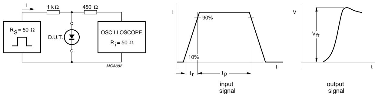
Fig.8 Forward recovery voltage test circuit and waveforms.
