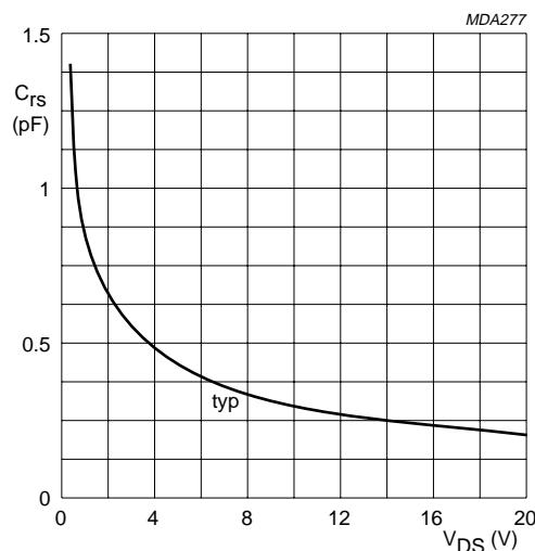
Fig.2  $V_{GS} = 0$  for BF410A and BF410B;
