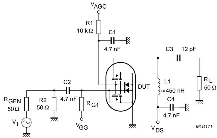
Fig.19 Cross-modulation test set-up.
