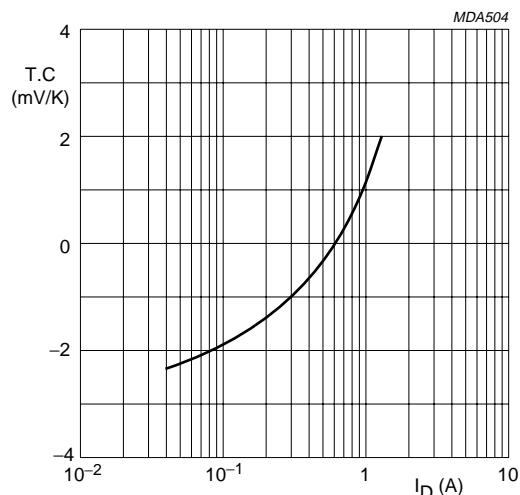
$V_{\text{DS}} = 10 \text{ V}$ .
