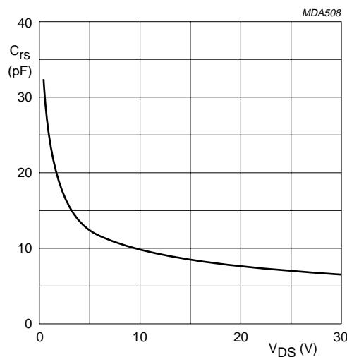
$V_{GS} = 0; f = 1 \text{ MHz.}$
