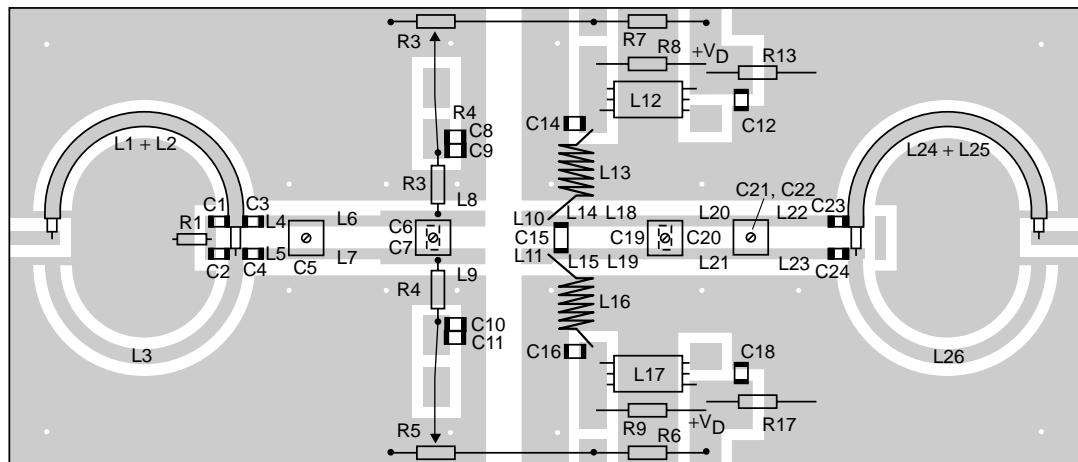
The circuit and components are situated on one side of the printed circuit board, the other side being fully metallized, to serve as a ground plane. Earth connections are made by means of copper straps and hollow rivets for a direct contact between upper and lower sheets.
