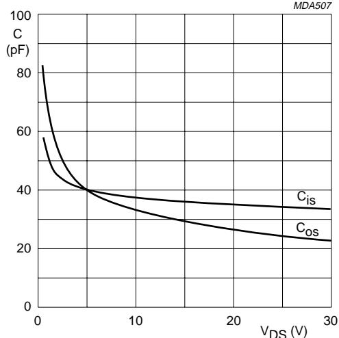
$V_{GS} = 0; f = 1 \text{ MHz.}$
