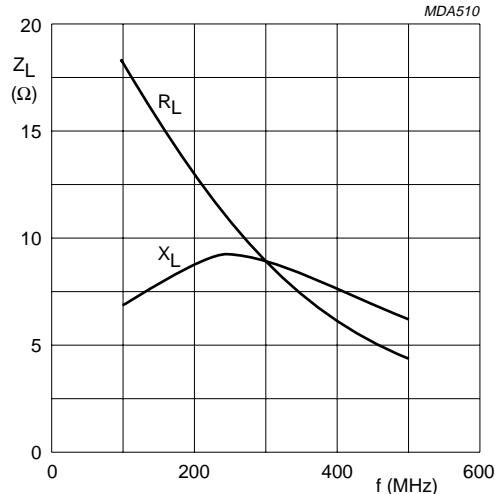
Class-B operation;  $V_{DS} = 28$  V;  $I_{DQ} = 2 \times 40$  mA;
