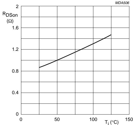
$I_D = 1.2 \text{ A}; V_{GS} = 10 \text{ V.}$
