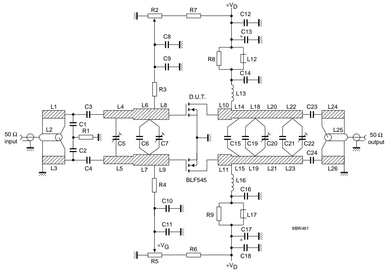
Fig.11 Test circuit for class-B operation.
