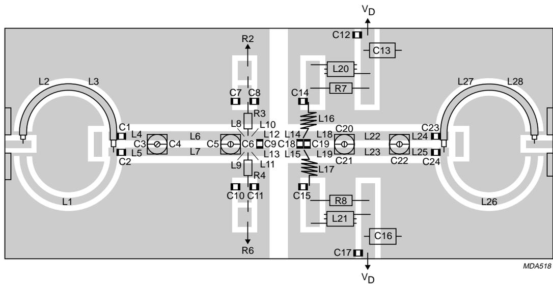
The circuit and components are situated on one side of the printed circuit board, the other side being fully metallized, to serve as a ground plane. Earth connections are made by means of copper straps and hollow rivets for a direct contact between upper and lower sheets.
