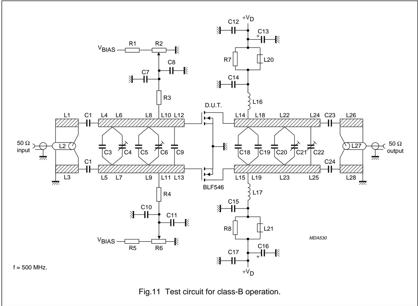
Fig.11 Test circuit for class-B operation.
