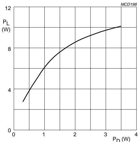
Class-B operation;  $V_{CE} = 7.5$  V;  $f = 470$  MHz.
