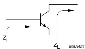
Fig.13 Definition of transistor impedance.
