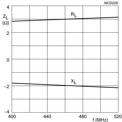
Class-B operation;  $V_{CE} = 7.5$  V;  $P_L = 8$  W.
