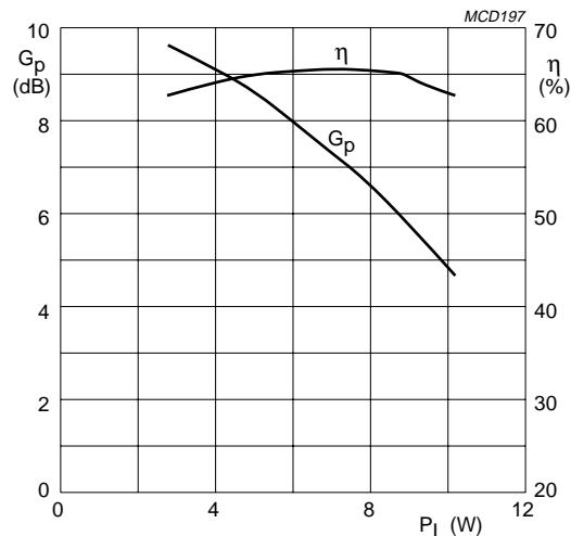
Class-B operation;  $V_{CE} = 7.5$  V;  $f = 470$  MHz.
