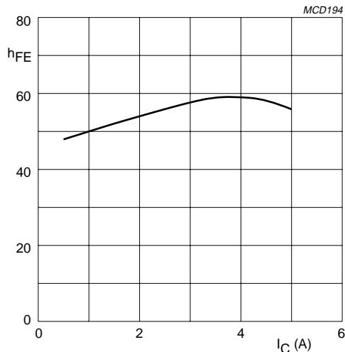
$V_{\text{CE}} = 5 \text{ V}$ .
