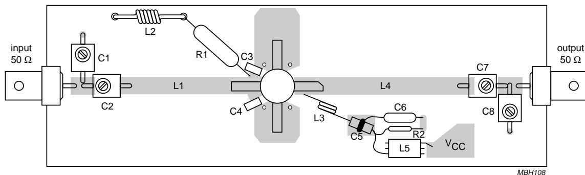
The circuit and components are situated on one side of a copper-clad PTFE fibre-glass board; the other side is unetched and serves as a ground plane. Earth connections from the component side to the ground plane are made by means of hollow rivets.
