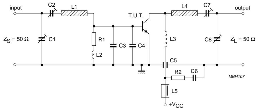
Fig.9 Class-B test circuit at  $f = 470$  MHz.
