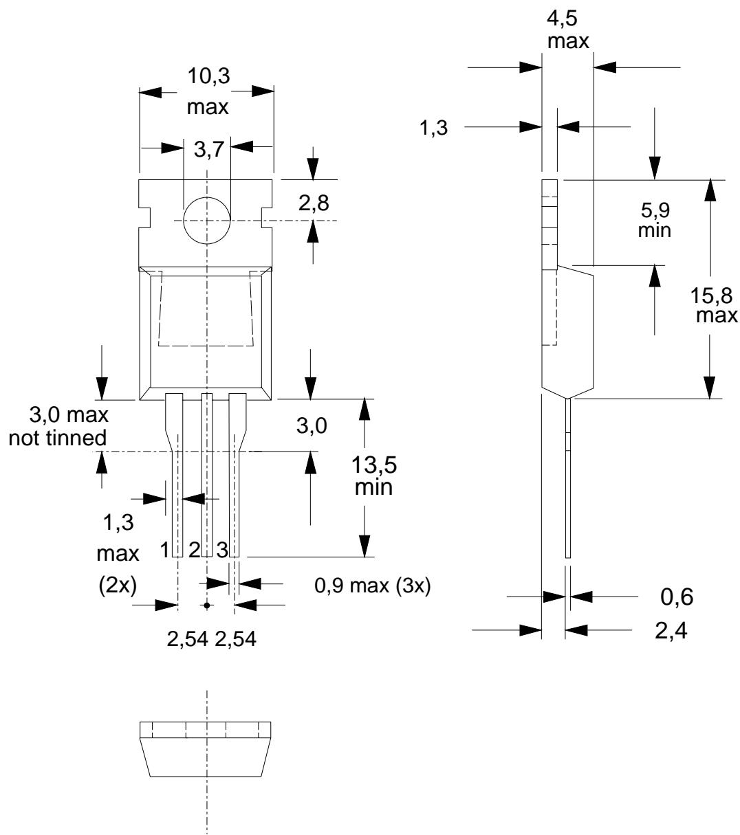
Fig.13. TO220AB; pin 2 connected to mounting base.
