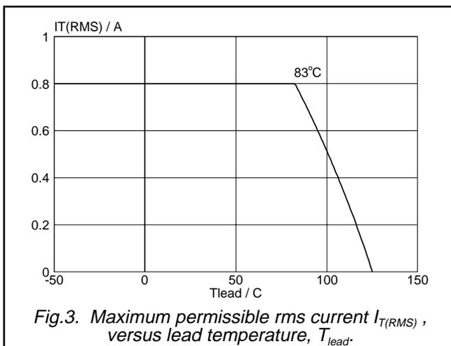
Fig. 3. Maximum permissible rms current  $I_{T(RMS)}$ , versus lead temperature,  $T_{lead}$ .
