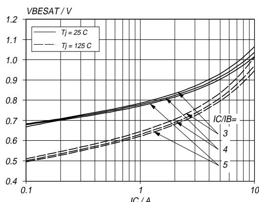
Fig.5. Typical base-emitter saturation voltage.
