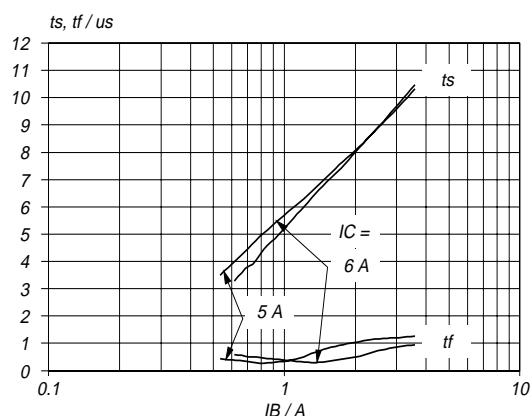
Fig.10. Typical collector storage and fall time.
