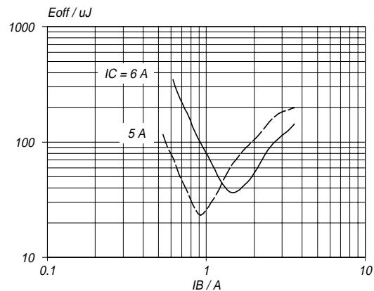
Fig.9. Typical turn-off losses.  $T_j = 85^\circ\text{C}$
