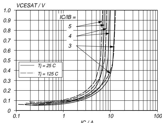
Fig.6. Typical collector-emitter saturation voltage.
