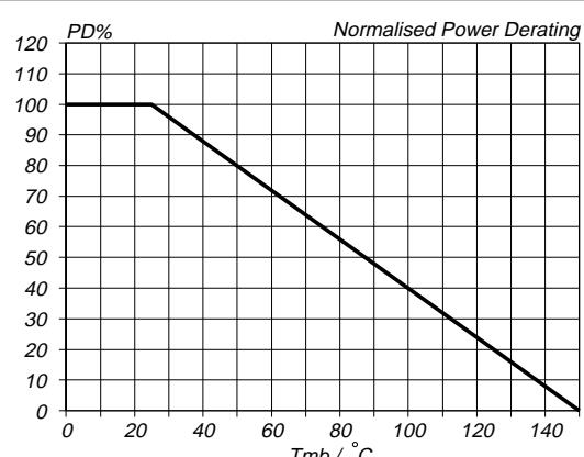
Fig.11. Normalised power dissipation.
