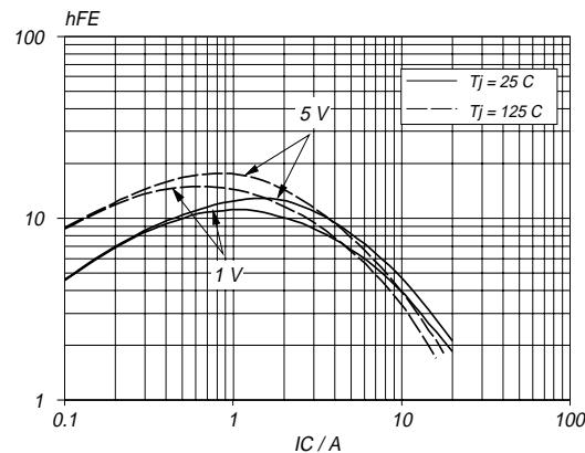
Fig.4. Typical DC current gain.  $h_{FE} = f(I_C)$
