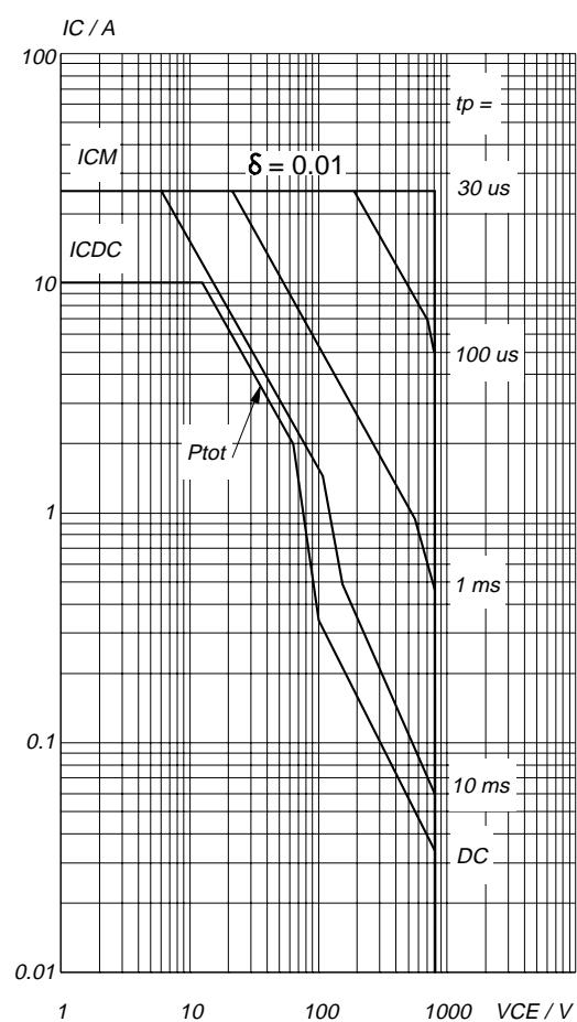
Fig.13. Forward bias safe operating area.  $T_{mb} = 25^\circ\text{C}$
