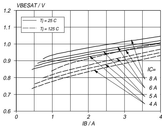
Fig.7. Typical base-emitter saturation voltage.
