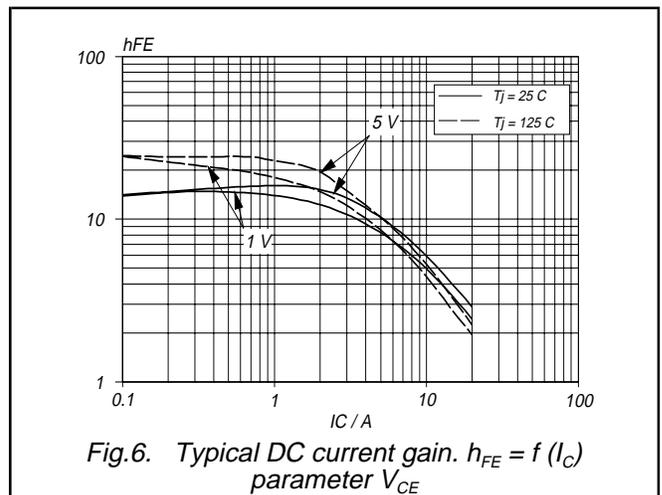
Silicon Diffused Power Transistor
