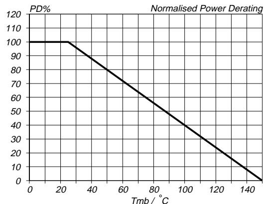
Fig.13. Normalised power dissipation.
