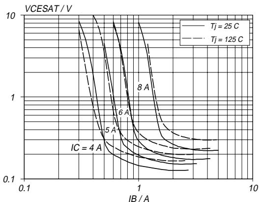
Fig.10. Typical collector-emitter saturation voltage.
