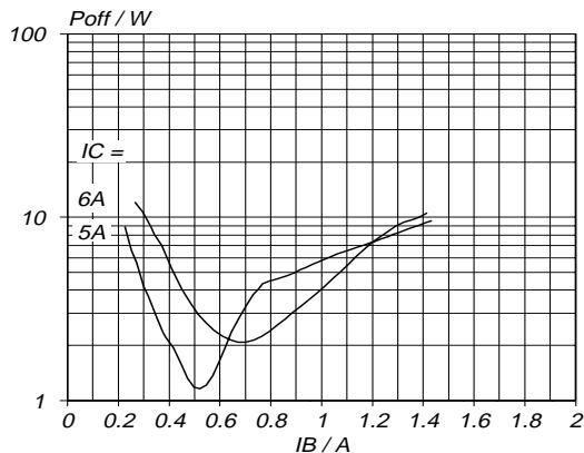
Fig.11. Typical turn-off losses.  $T_j = 85^\circ\text{C}$
