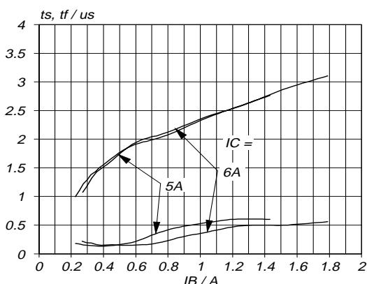
Fig.12. Typical collector storage and fall time.
