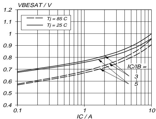
Fig.8. Typical base-emitter saturation voltage.
