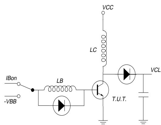
Fig.16. Test circuit RBSOA.  $V_{CC} = 150 V$ ;  $-V_{BB} = 5 V$
