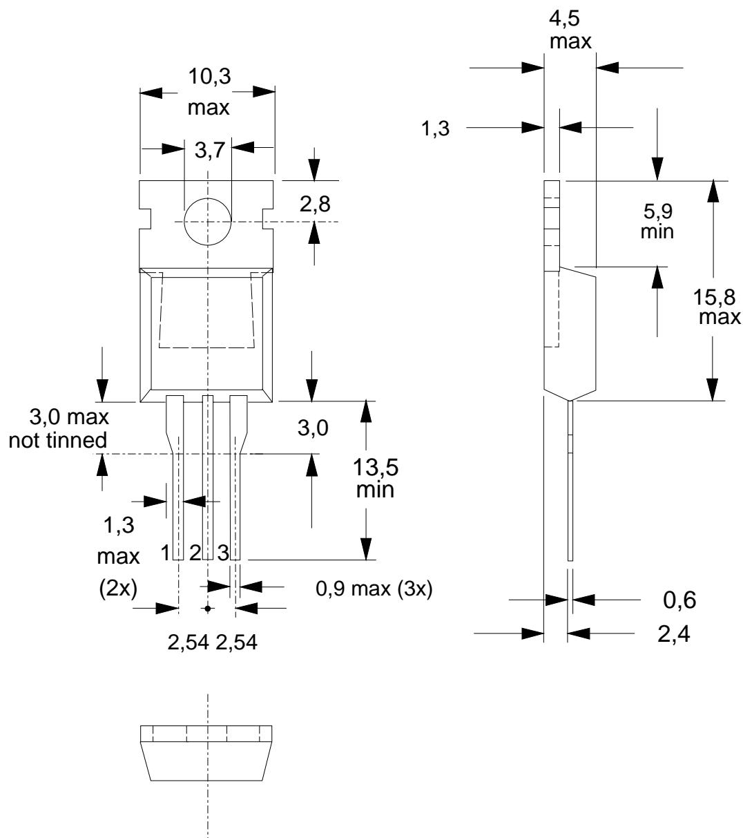
Fig.17. TO220AB; pin 2 connected to mounting base.
