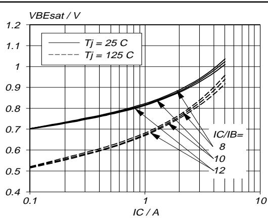
Fig.9. Typical base-emitter saturation voltage.
