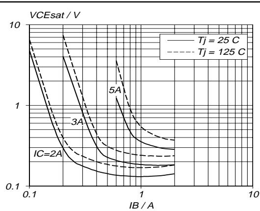
Fig.12. Typical collector-emitter saturation voltage.
