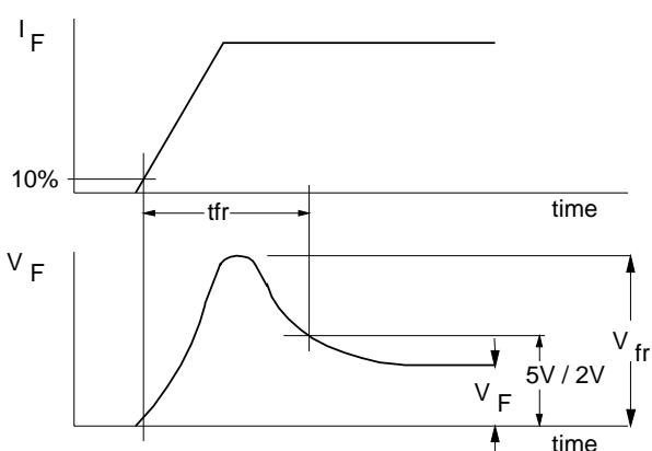
Fig.1. Definition of  $V_{fr}$  and  $t_{fr}$
