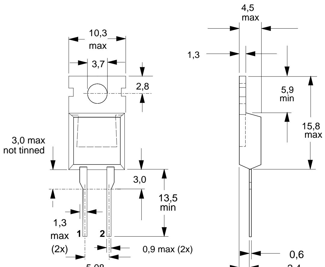
Fig.7. SOD59 (TO220AC). pin 1 connected to mounting base.
