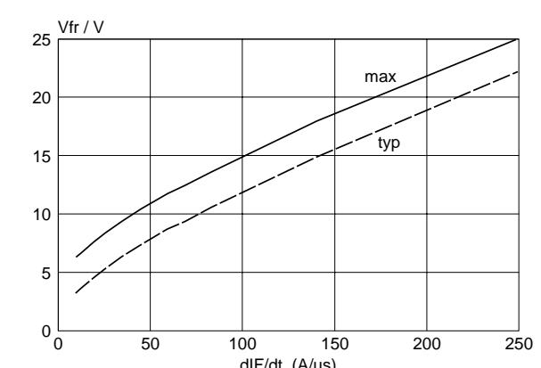
Fig.5. Typical and maximum  $V_{fr} = f(dI_F/dt)$ ;  $I_F = 10 \text{ A}$ ;  $T_j = 25^\circ\text{C}$
