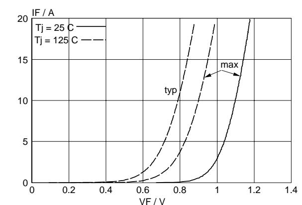
Fig.4. Typical and maximum forward characteristic
