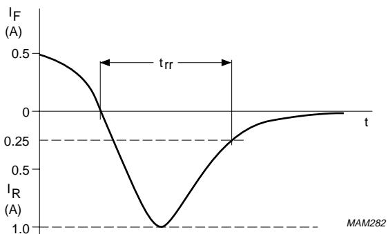
Fig.10 Test circuit and reverse recovery time waveform and definition.
