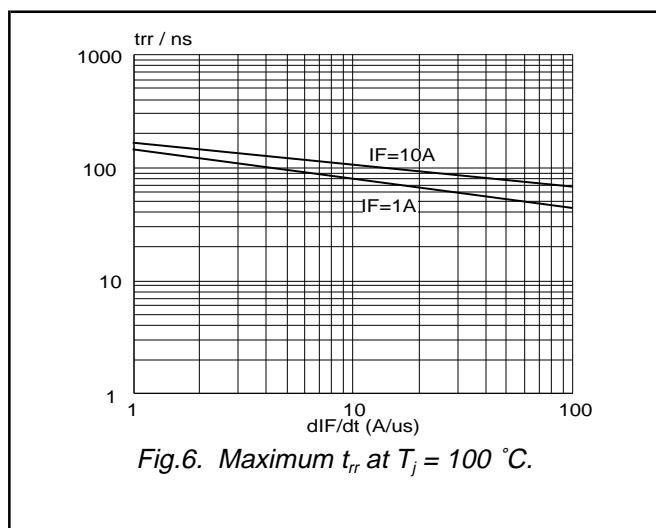
Fig.6. Maximum  $t_{rr}$  at  $T_j = 100$  °C.
