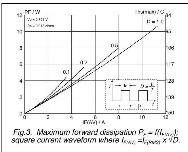
Fig.3. Maximum forward dissipation  $P_F = f(I_{F(AV)})$ ; square current waveform where  $I_{F(AV)} = I_{F(RMS)} \times \sqrt{D}$ .
