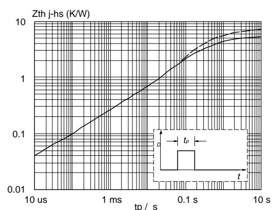
Fig.11. Transient thermal impedance;  $Z_{th j-hs} = f(t_p)$ .
