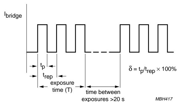
Fig.9 Maximum current through a 3-phase bridge rectifier versus pulse duration; exposure time  $T = 1$  s;
