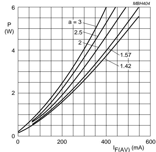
$$a = I_{F(\text{RMS})}/I_{F(\text{AV})}; \delta = 0.5; V_R = V_{RW\text{Mmax}}$$
