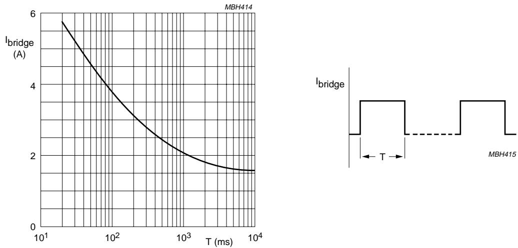
Fig.8 Maximum permissible output current in a 3-phase rectifier bridge with a minimum time between exposures of 20 s;  $T_{\text{oil}} = 50^\circ\text{C}$ .
