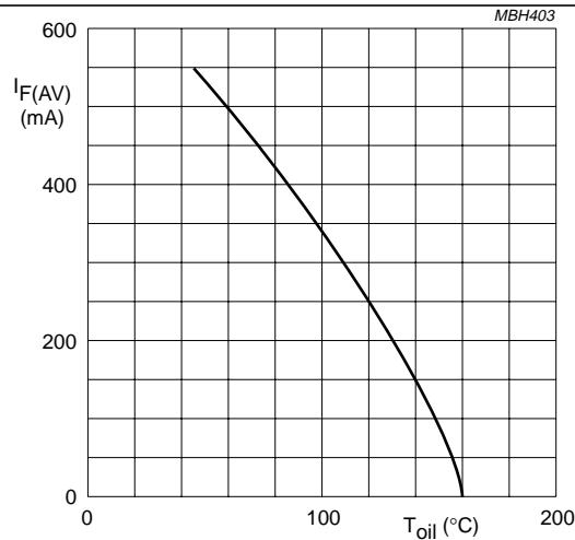
$$a = 1.57; \delta = 0.5; V_R = V_{RW\text{Mmax}}$$
