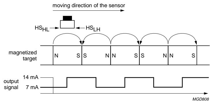
Fig.3 Functional principle of KMI15/2.
