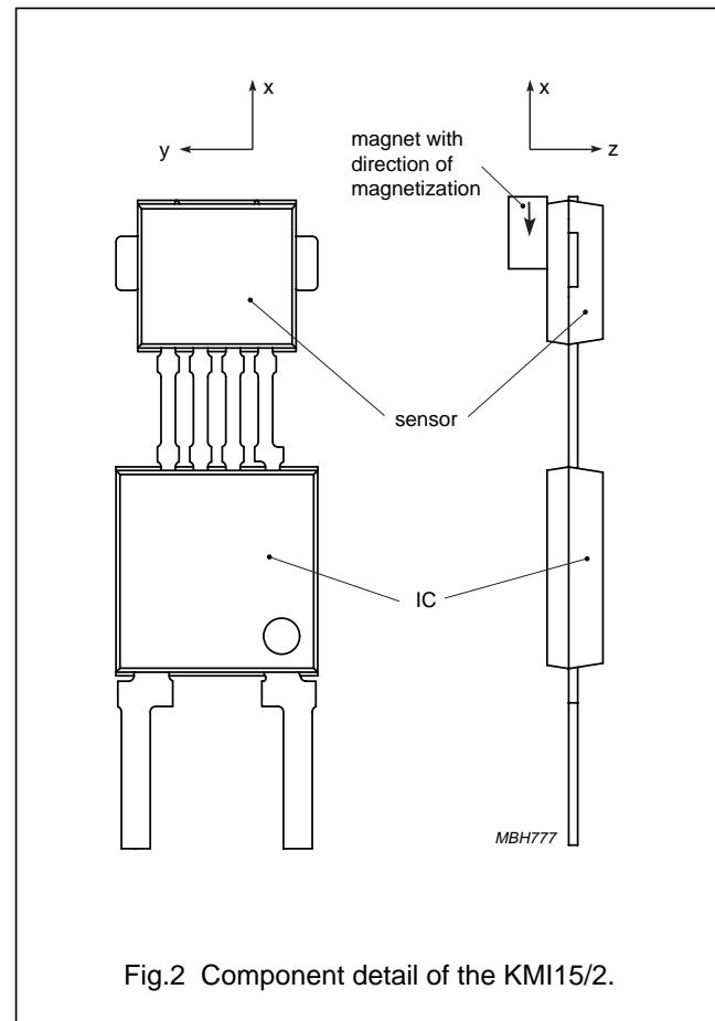
Fig.2 Component detail of the KMI15/2.
