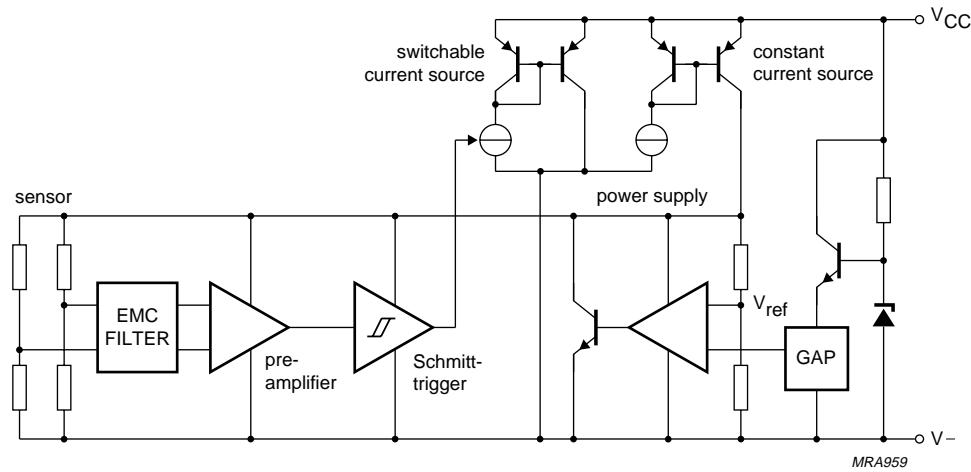
Fig.5 Simplified circuit diagram.
