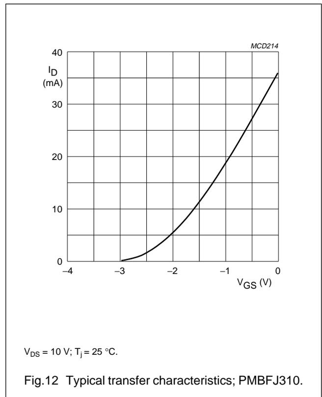
N-channel silicon field-effect transistors
