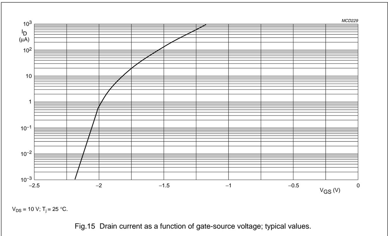
N-channel silicon field-effect transistors
