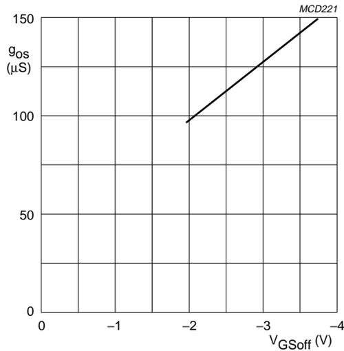
$V_{DS} = 10 \text{ V}; I_D = 10 \text{ mA}; T_j = 25 \text{ }^\circ\text{C}.$
