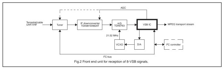
Symbol timing recovery is performed mostly within the VSB IC, except that a low cost D/A converter and VCXO are required externally to generate the nominal 21.52 MHz clock for the A/D converter and VSB IC.
