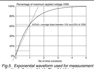
Fig.5. Exponential waveform used for measurement of critical off-state  $dV_D/dt$ . The  $dV_D/dt$  is the average slope between 10% and 63% of the maximum applied voltage  $V_{DM}$ .
