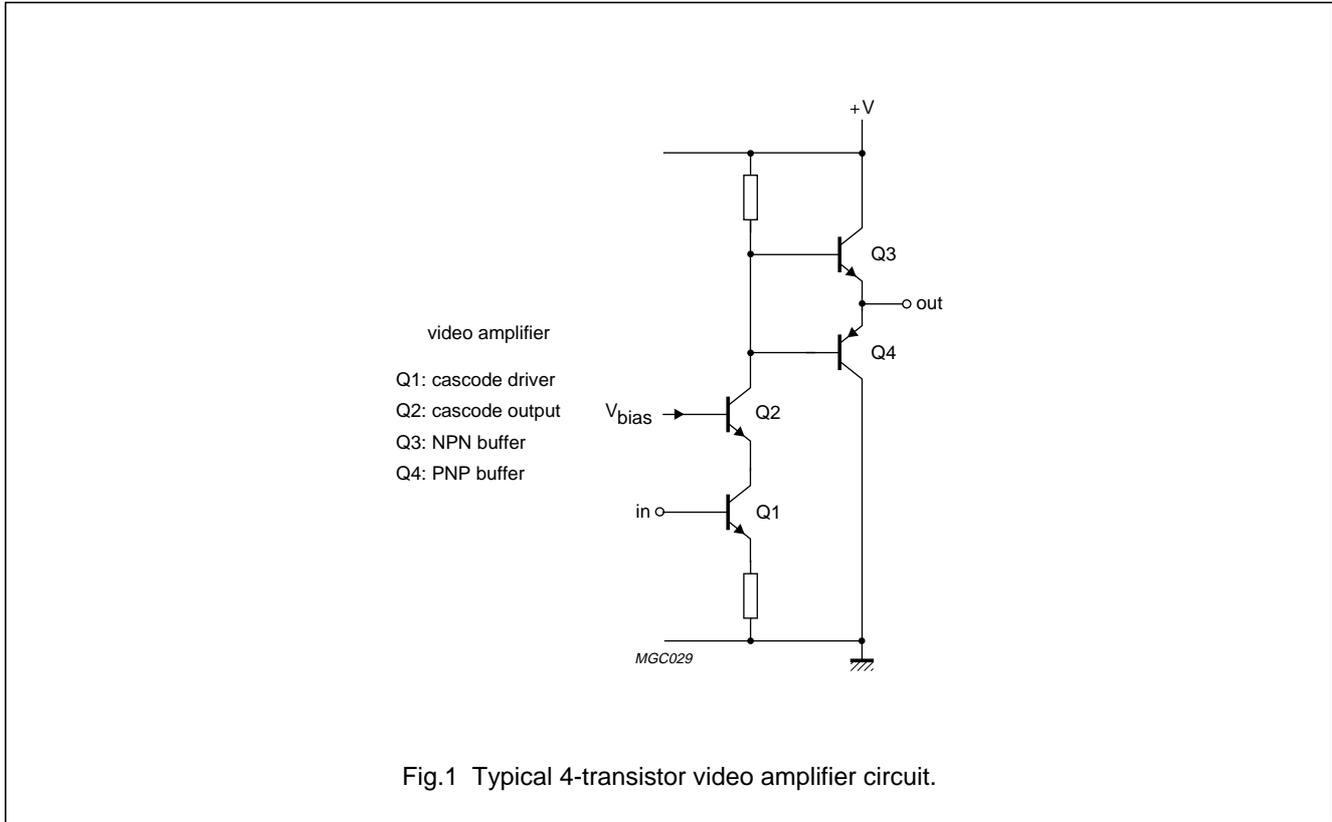
Fig.1 Typical 4-transistor video amplifier circuit.
