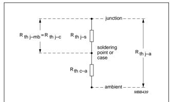
Fig.2 Representation of thermal resistance paths of a device mounted on a substrate or printed board.
