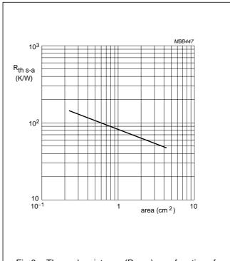
$\label{eq:Fig.8} Fig. 8 \quad \text{Thermal resistance } (R_{\text{th s-a}}) \text{ as a function of area of ceramic substrate.}$
