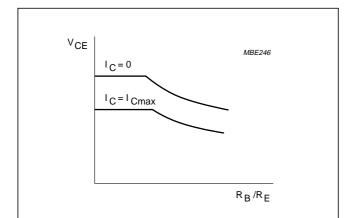
Fig.2 Graph showing effect of collector current on permissible operating areas.
